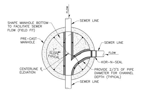
NOTE: SEE PLAN 411 R DRAWING 2 OF 2 FOR BASE TYPICAL BASE CONFIGURATIONS.
